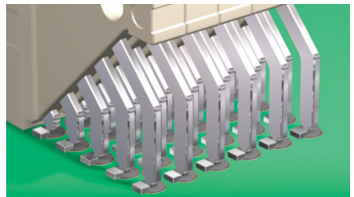
Preforms provide additional solder for tight pitch components and thick PCBs ensuring 100% hole fill and fillet formation.
