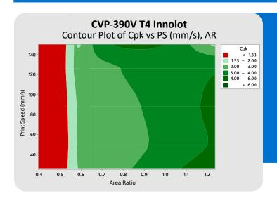
ALPHA CVP-390V maintains >1.66 Cpk for transfer efficiencies between 60%-120% on AR ≥ 0.6 across all print speed process conditions.
