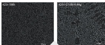
Figure 1. Microstructure of 42Sn-58Bi and 42Sn-57.6Bi-0.4Ag
