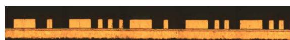
Systek™ ETS embedded trace filling with excellent thickness distribution, plating to replace filling.
