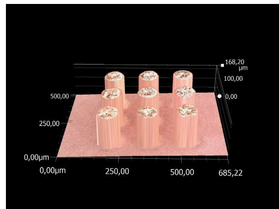
Figure 22. Impression of Pillar Plating works
