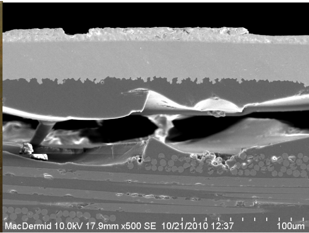
Fig. 6 – Delamination After Reflow
