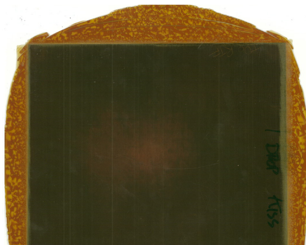
Fig. 4 - Resin Bead with Moisture
