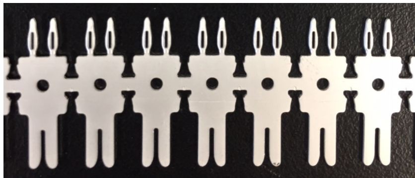
The M-Contact IN-2000 plates a uniform indium coating over complex shapes.
