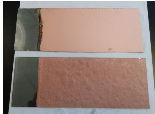
Figure 3. Films produced on polished stainless steel substrates for elongation testing. Top - stress free copper deposit from the new high build electroless copper system Bottom - Conventional high build electroless copper.
