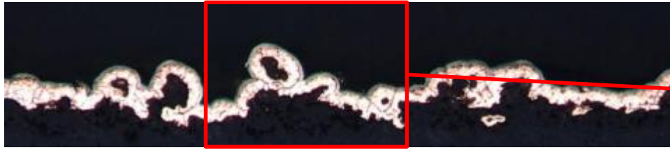
Cu grain structure after peroxide etch. Light Adjusted for Plastic
