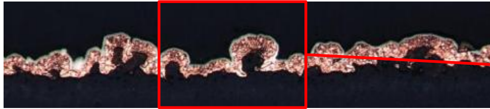
Cu grain structure after peroxide etch.
